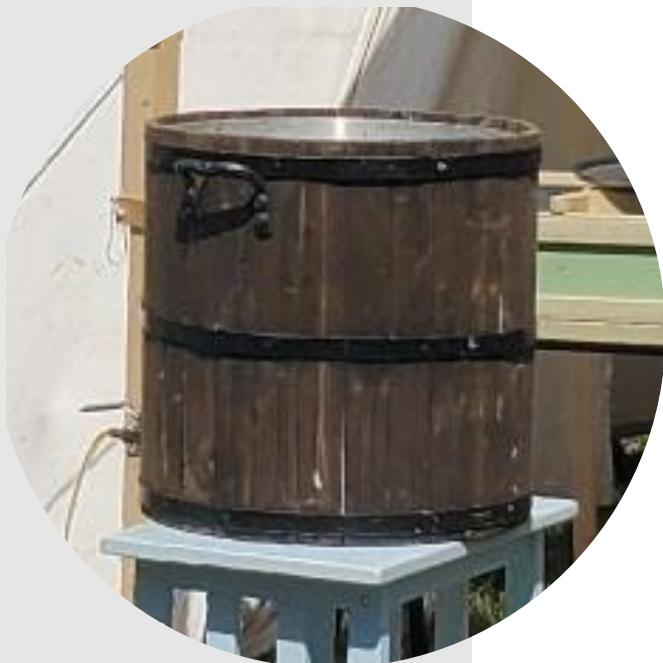
A kieve is a tub or vat used to mash and subsequently lauter wort. The term comes from the German word *kübel* which means bucket and my kieve is just that, a large (30 gallon to match the copper) bucket with wooden sheathing to keep in the heat.
